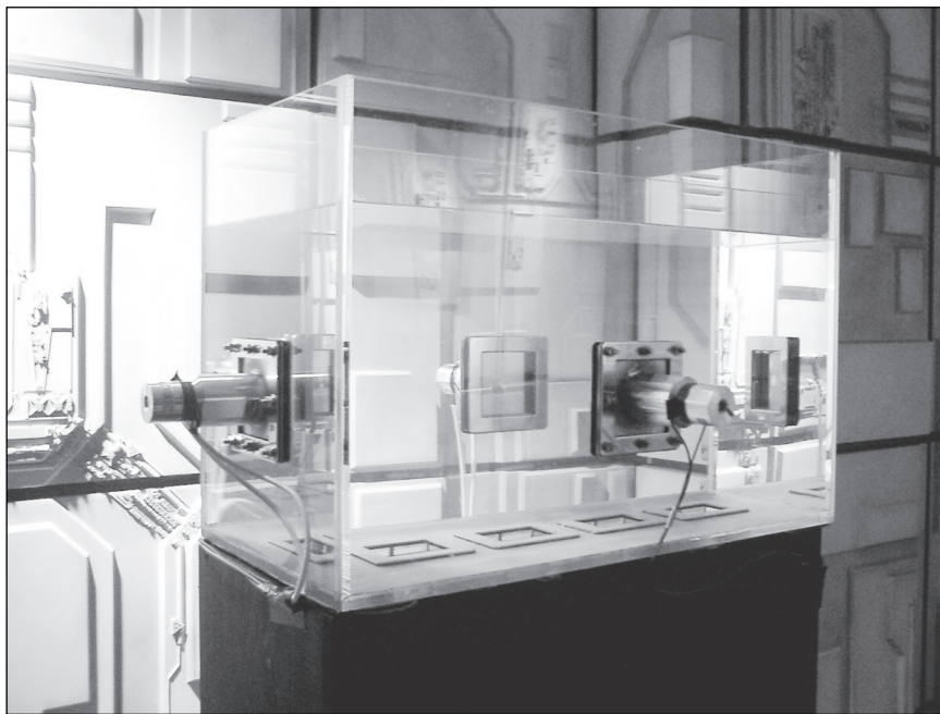
Fig. 4. Transparent chamber (60×40×30 cm) with eight ultrasonic transducers custom-designed by Honda Electronics: four on the sides and four at the bottom. (Photo © Evelina Domnitch and Dmitry Gelfand)
