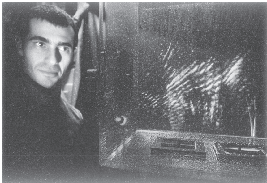
Fig. 3. Six-channel Camera Lucida prototype: A 20–10-kHz signal irradiates a solution of luminol and ammonium sulfate, resulting in parallel lines of sonoluminescence corresponding to the troughs of the sound waves. (Photo © Chunichi Shimbun)
